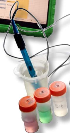
pH is measured using a pH meter and probe.
