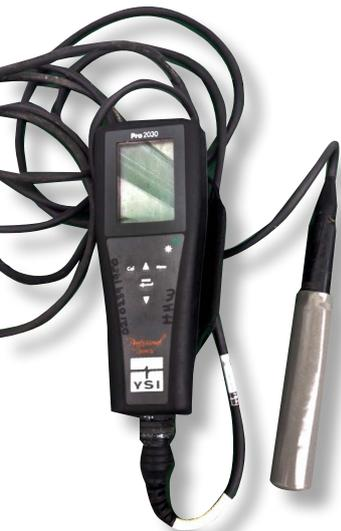
PRO2030 Instrument for measuring water temperature, DO, electrical conductivity
